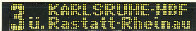
Righth-hand side: Single display for number and destination VDV-STÜLB window: 220 x 1400 mm (H x W), area and dot size as front.
