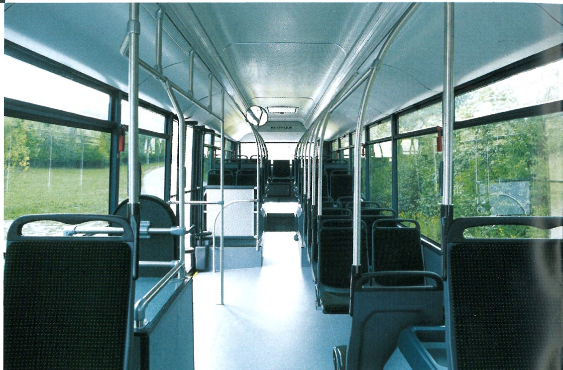
Practical: The cantilever mounting of the seats, fitted on side-wall rails.
