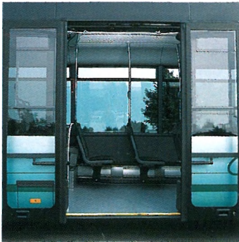
Entrance without obstacles – the Centroliner's middle door with no steps.
