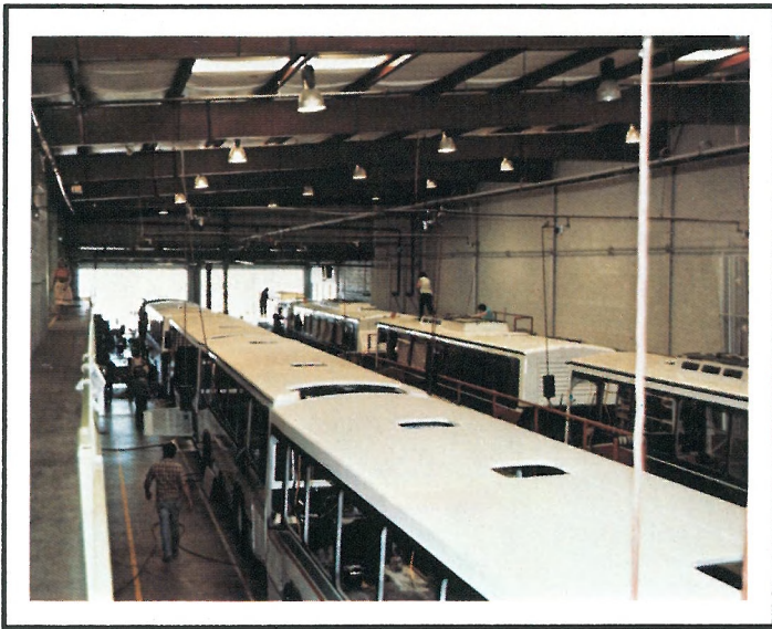
In the final finishing area, all interior components such as seat, drive trains, air conditioning, flooring, insulation, trim panels, etc., are installed.
