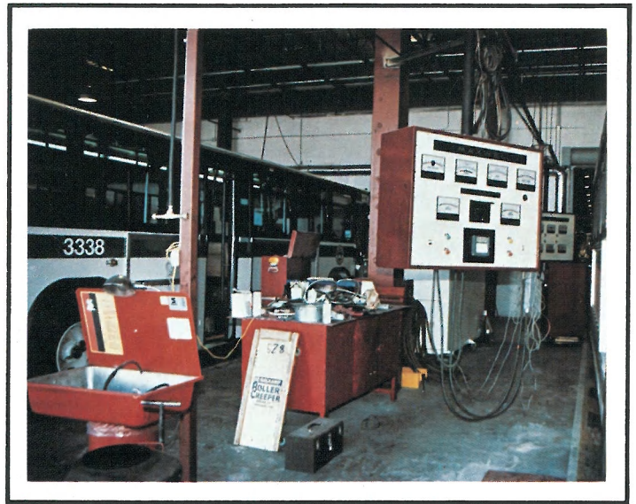
NEOPLAN performs a complete dynamometer test on every vehicle before shipping to the final destinations.
