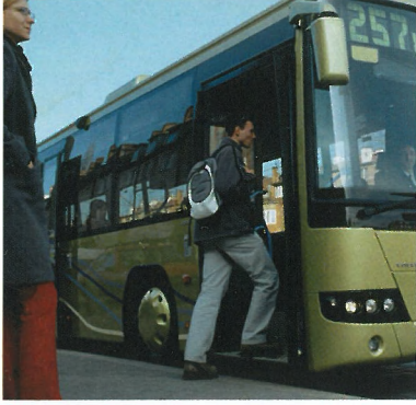
Boarding height at the front is 320 mm and this can be lowered a further 90 mm with the kneeling function.
