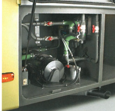
The Volvo 8700 Low Entry can be equipped with an auxiliary heating system.
