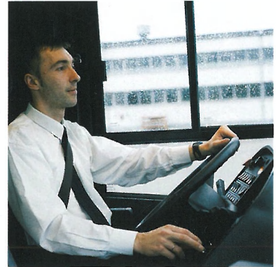
The instrument panel moves with the steering wheel when this is adjusted, so you always have the instruments at the correct distance and angle.
