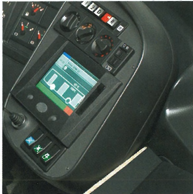
Information from the bus's electronically controlled functions is shown in a display unit.
