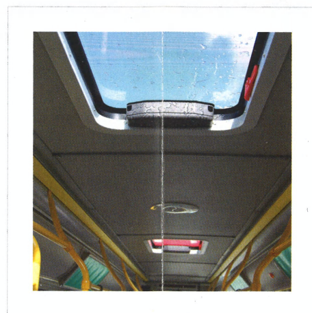
Transparent and electrically controlled roof windows for interior brightness
