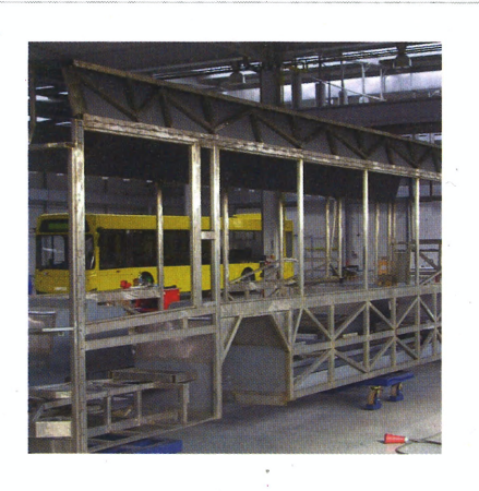
Bodywork frame of stainless steel = long life span period of the vehicle
