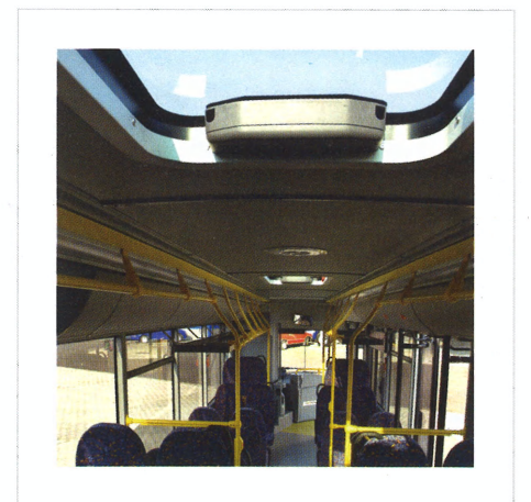
Transparent and electrically controlled roof windows for interior brightness
