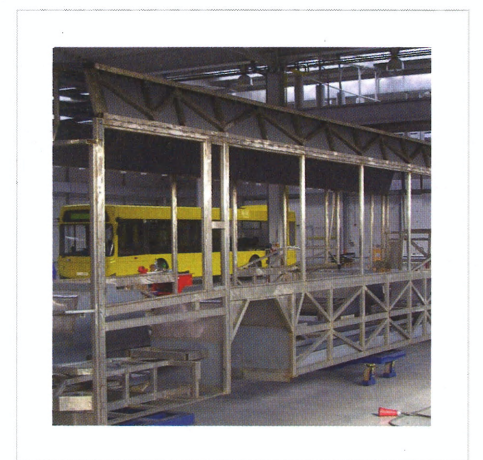
Bodywork frame of stainless steel = long life span period of the vehicle
