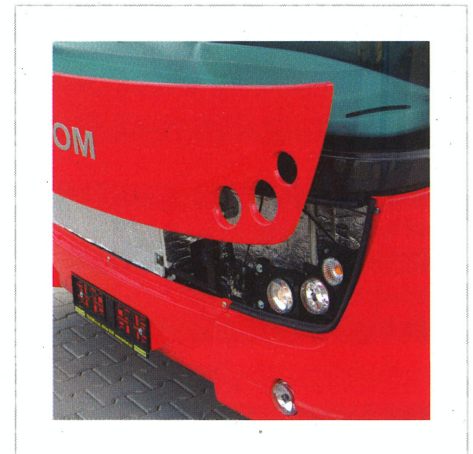
Easy access when lights replacing
