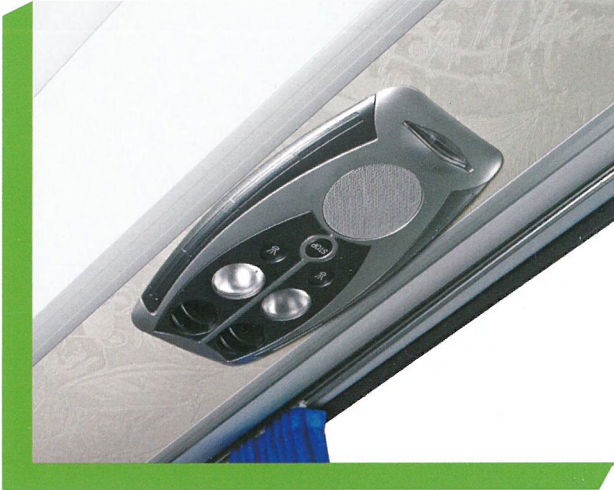
Concealed air-conditioning outlet combined with illumination light makes warmth and comfort.
