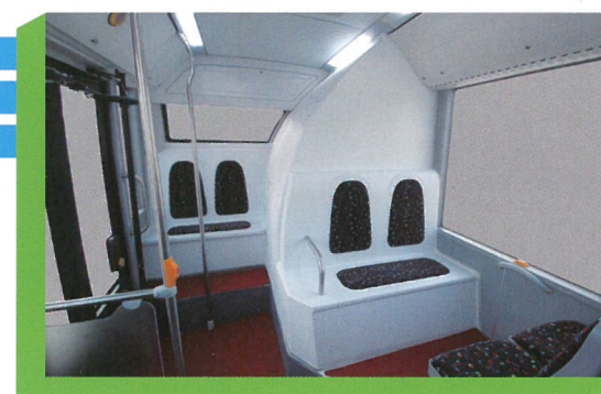
Side placement of engine makes it possible to adopt low floor design and offer quick boarding & alighting experience.
