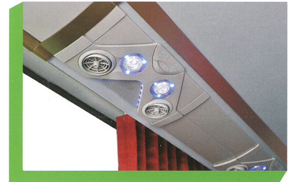
Integral design of reading lamps, air conditioner outlets, trim with human-oriented and considerate concept.
