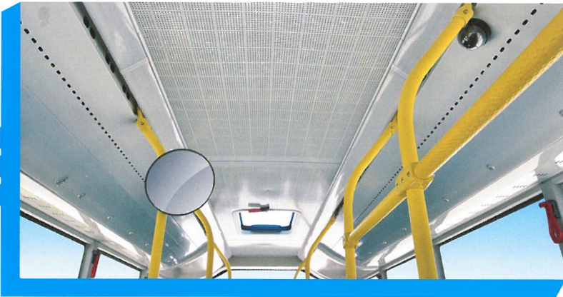
Molding aluminum interior roof and KING LONG roof-mounted dependent air conditioning system provides intelligent temperature control.
