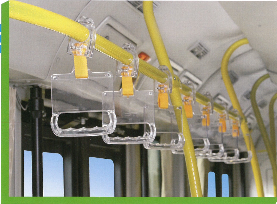
Suspended strap handles, at a proper height, ensure more safety for standing passengers.
