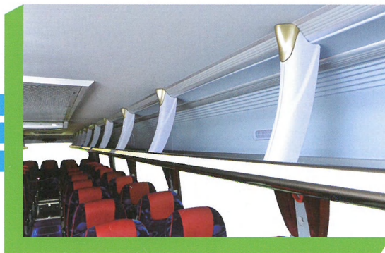
Luggage rack tilting design preventing luggage from falling down and night lamp for night operation which is human-oriented.
