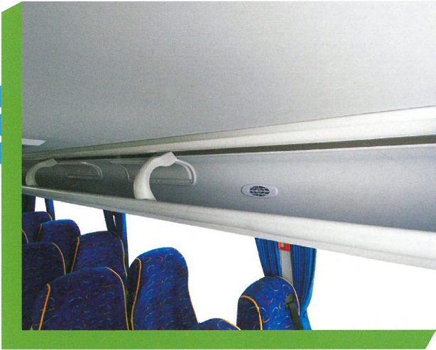
Luggage rack tilting design can prevent luggage from falling down, and with blue night lamp for night operation which is friendly for using.
