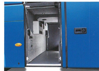
The baggage compartment is specially designed with a driver room for sleeping, with visual window and airconditioning.
