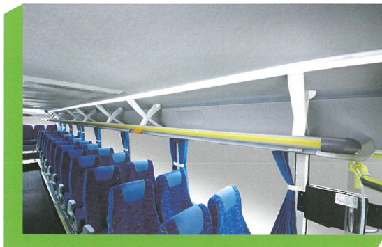
Luggage rack in brand new style has a volume of 1.5m . High-capacity makes convenience.
