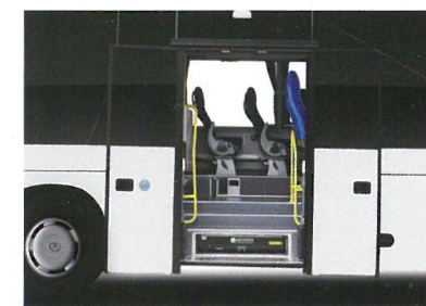
Unique double swinging middle door effectively improves passenger flow rate. Wheelchair lifting device provided as option.
