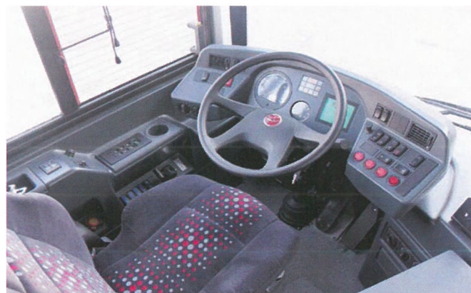
Sileo has an ergonomic VDV workstation in its currently available form. In the series, it will receive its successor, developed by Continental, in which the consumption data is displayed in the dash panel.
