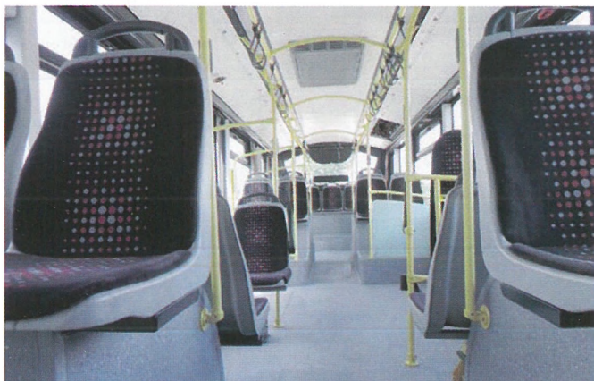
Our test bus has 32 seats available; the total capacity is just under 90 people. By eliminating the engine compartment, rear left, a second special use area can be incorporated.
