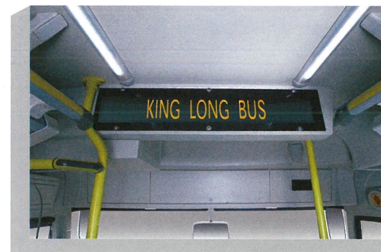
LED interior destination plate with stop alert function.
