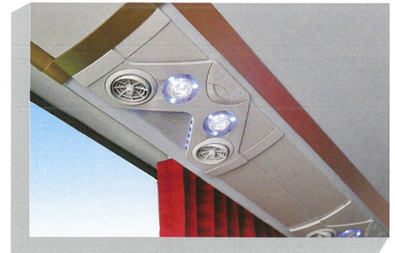
Equipped with reading lamps and A/C outlets.
