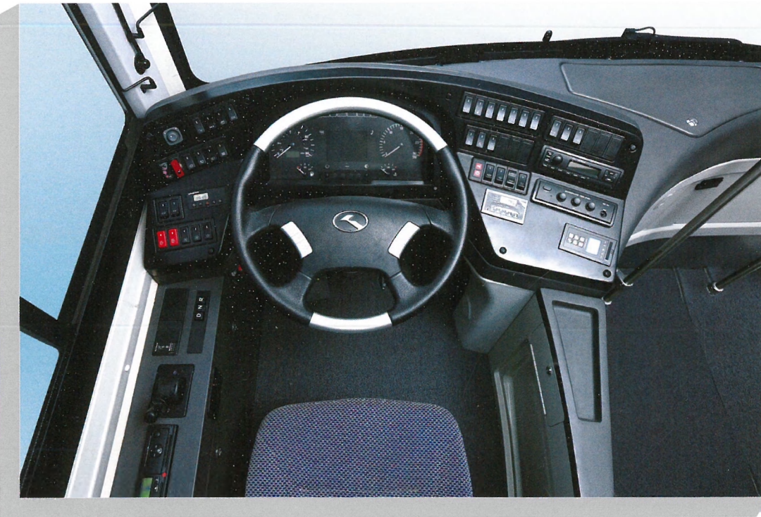
Integrated instrument panel with complete functions for more convenient operation.
