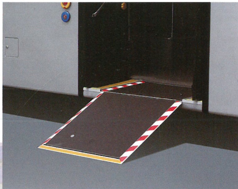
Automatic lifting/lowering foot-step is optional set up in middle door, easy for disabled to get on and off.
