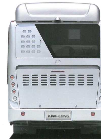
Unsymmetrical design of the rear windshield helps dissipate heat from engine.
