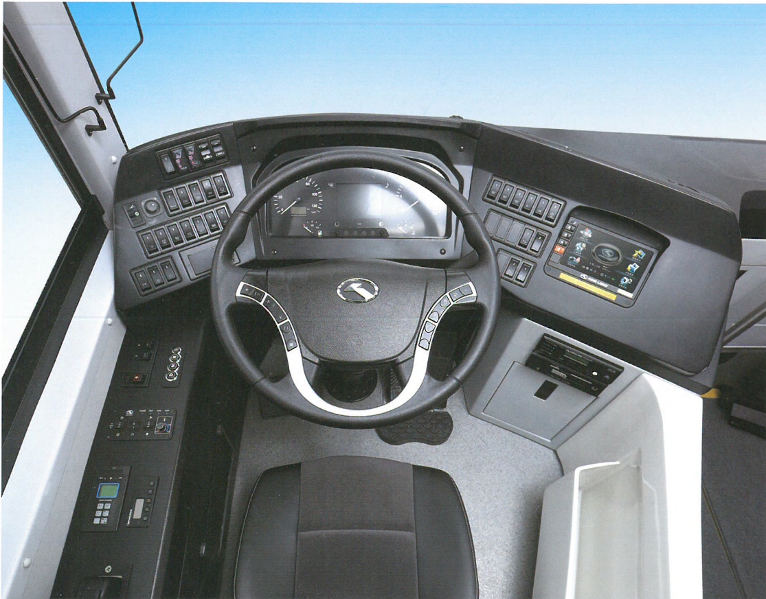
King Long multi-functional steering wheel is integrated with buttons of electric appliances, makes it easier for the driver to control.
