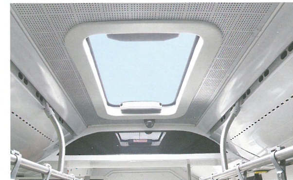
Sunroof in the front and the rear roof give passengers more daylighting.
