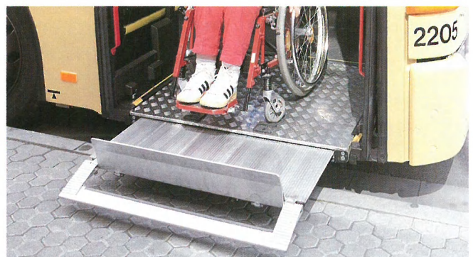
The front entrance can be equipped with a lifting platform for wheelchair users. ▼
