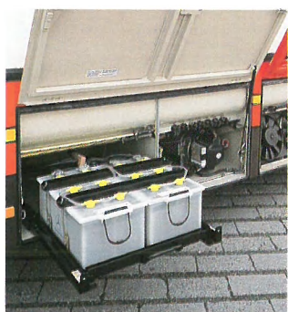
The batteries are mounted on extendable frames to permit rapid checks on their condition.
