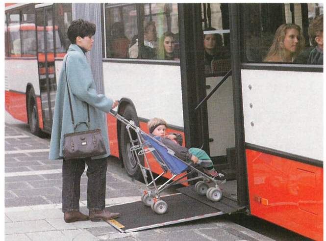
The front entrance can be equipped with a lifting platform for wheelchair users. ▼
