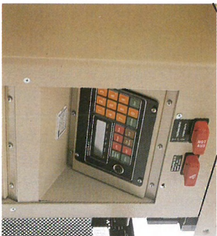
The controls for the destination signs are located above the driver's seat.
