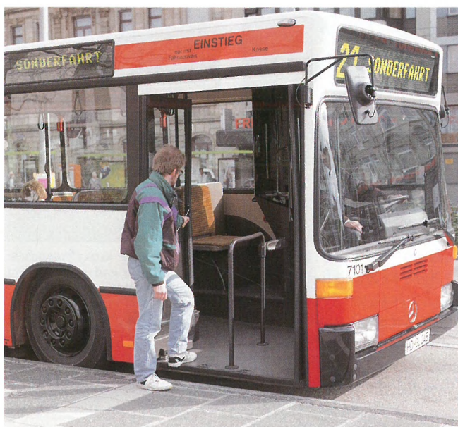
The low entrance height of just 317 mm at the front door and the double-wing inward-swinging doors make access easier.
