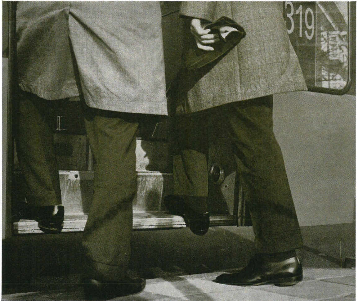
The wide, easy entrance cuts waiting time at bus stops. This is particularly so when dual flow entry is adopted, separating passengers already in possession of a ticket from those who have to purchase a ticket from the driver. The low entrance height is very noticeable.
