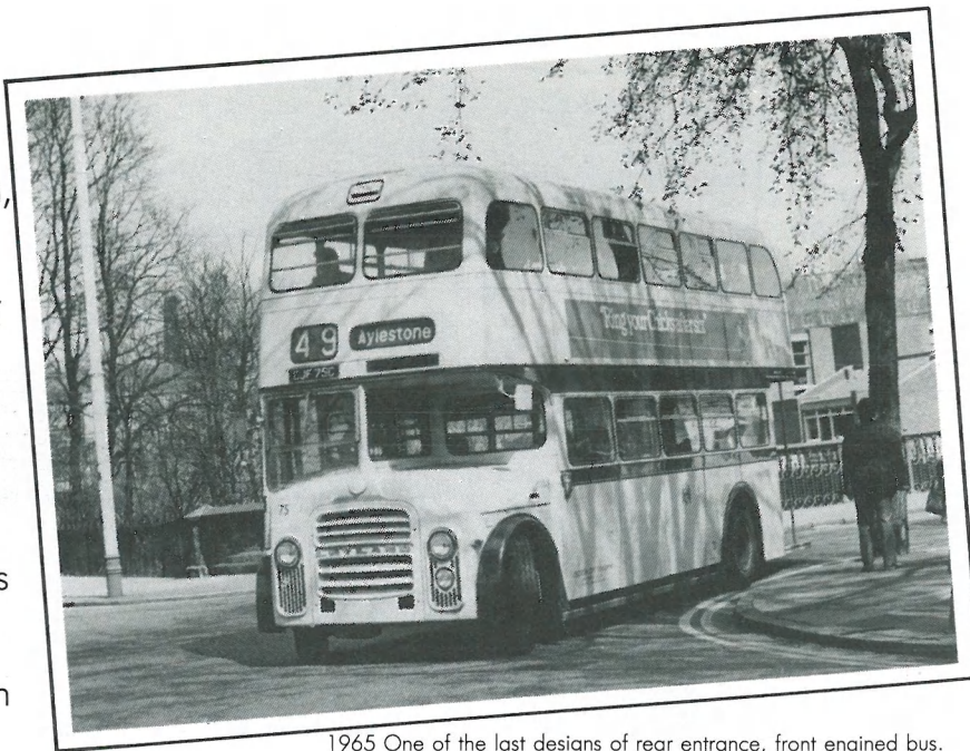
1965 One of the last designs of rear entrance, front engined bus. This Leyland Titan PD3 No 75 was withdrawn in 1980
