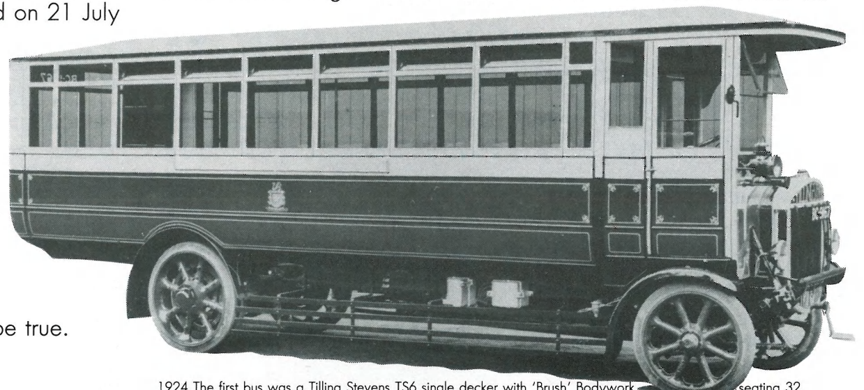
1924 The first bus was a Tilling Stevens TS6 single decker with 'Brush' Bodywork seating 32
