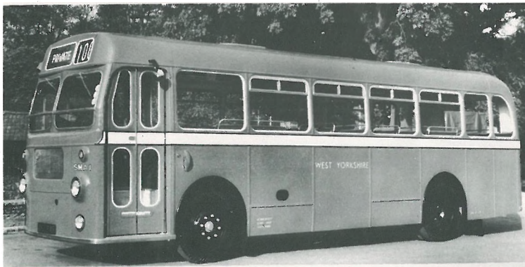
Bristol/ECW small capacity 36-seater bus on SU type chassis currently in production.
