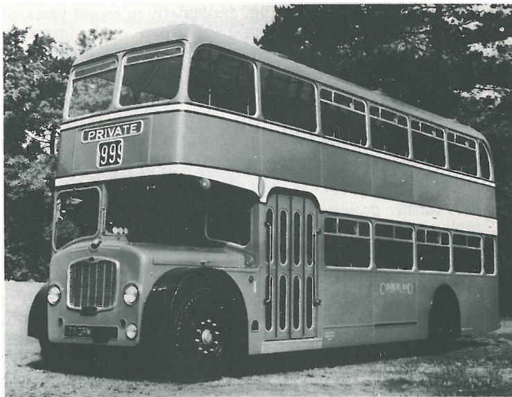
Bristol/ECW F.L.F. type 70 seater stepless forward entrance flat floor Lodekka bus.
