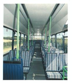
the whole image of bus travel. A variety of modern seat designs can be fitted and a typical interior layout provides space for up to 52 seated passengers plus 23 standees.
