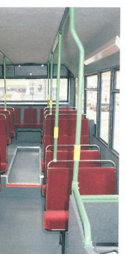
between 35 and 43. Seating layouts can be varied to meet specific requirements and include the option of single seats near the front of the vehicle to maximise circulating space. A luggage pen can be fitted over the front wheelarch and high-backed coach seats can be supplied for added passenger comfort.
