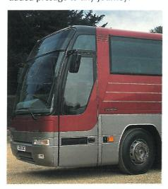
The wide entrance has a plug door, manufactured to strict tolerances using RTM and installed to fit tightly to cut noise.
