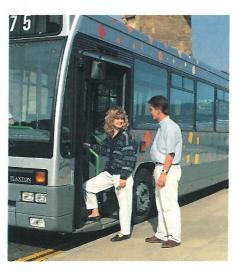
The split-step entrance and wide doorway makes boarding and alighting easy. The floor on each chassis variant has been designed to make passenger movement as safe and easy as possible. The unobstructed floor makes cleaning easier, saving time and money.
