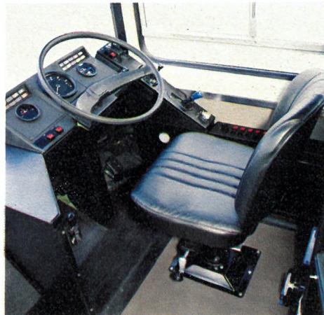
Ergonomically planned driving compartment with prioritized controls
