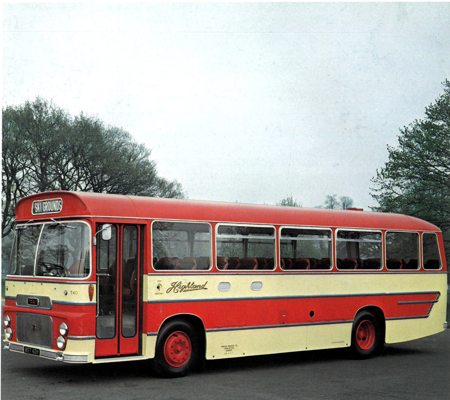
Above: Front-entrance 45-passenger PAYE bus on Ford R 192 chassis built for Highland Omnibuses Ltd. of Inverness.
