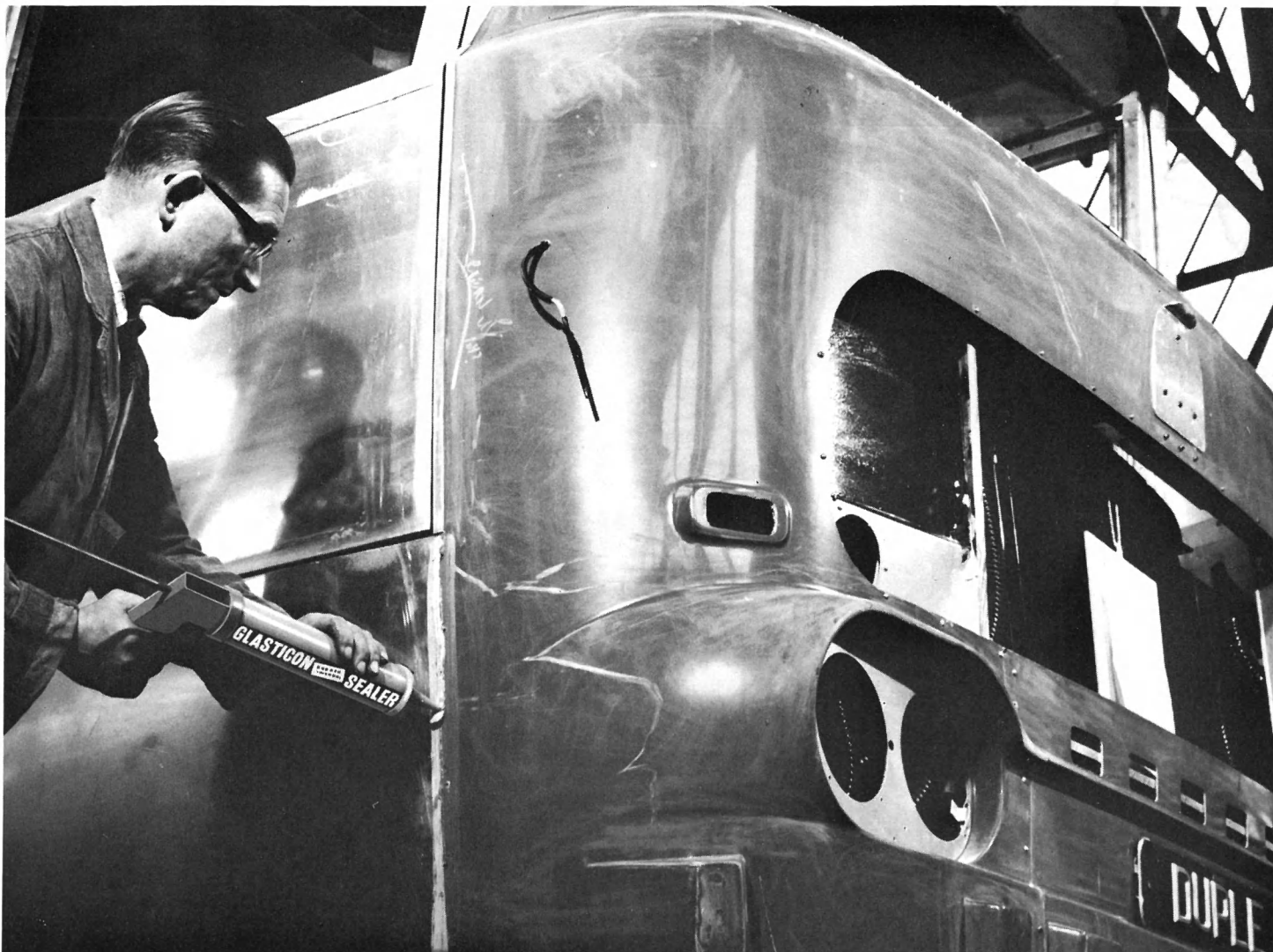
Photograph by kind permission of Duple Motor Bodies Ltd. illustrating joint application of Glasticon Gun Mastic.
