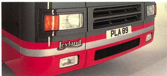
Sleek new front fibreglass grille and panelling in body colour with heavy duty bumper corners.
