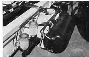
Dual air-over-hydraulic brakes; 20% greater brake area
