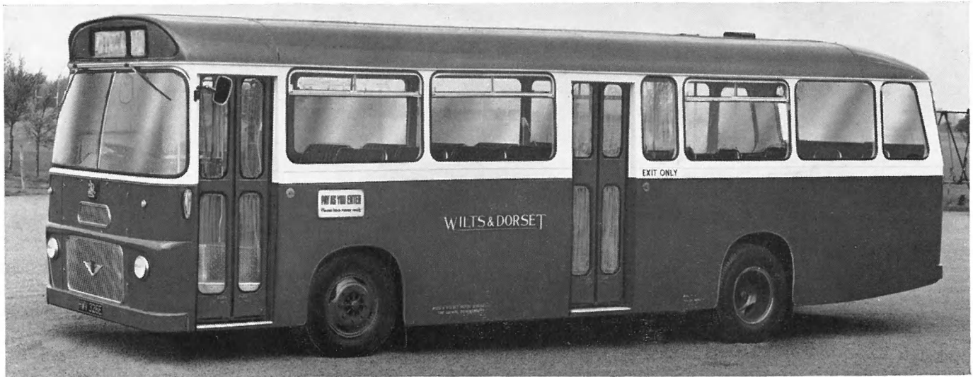
Hants & Dorset Single Decker FRONT ENTRANCE AND CENTRE EXIT REDRO SINGLE FOLDING DOORS ELECTRICALLY OPERATED. Bodied by Willowbrook Limited (Member of the Duplex Group)
