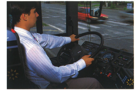
Functional and spacious driver's station. The instruments in the centre of the driver's field of vision.
