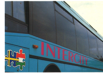
Glued side windows with flat body sides – elegant design and easy to keep clean.
