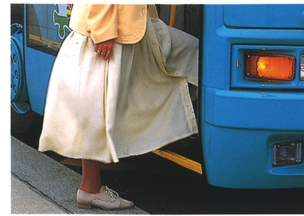
Low and convenient entrance step – with kneeling only 255 mm!
