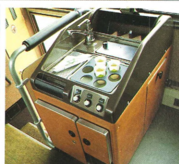
A demanding travelling public expects on-board catering as well – a good reason for fitting a galley either built-in, with water-heater and grill, or freestanding, with a refrigerator, behind the centre entrance.
