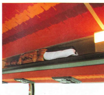
The luggage rack above the seats – harmoniously blended into the interior design – offers ample room for hand luggage. Interior and night lights and – if specified as an optional extra – loudspeakers are integrated into the shelf brackets.
