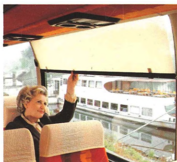
The roller blinds can be raised or lowered to any position to provide protection from sun and heat. The large arched side windows give an unrestricted view to all sides. (Double glazing is optionally available).
