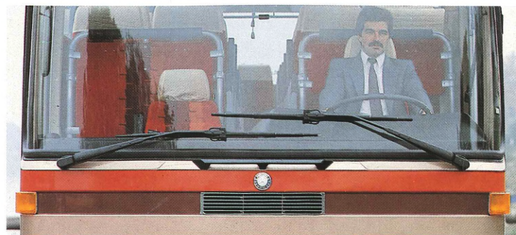
Synthesis of styling and function: the deep single-pane front windscreen with screen wipers at the bottom
