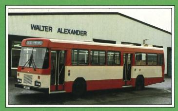
A prototype on the B60 chassis is illustrated and production units will be available following extensive vehicle development and proving trials including a Pave test.
