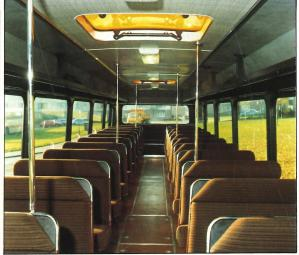
The Dual purpose "N" Type on the Leyland Tiger chassis features 53 dual purpose nylon trimmed seats with shoulder pads, flat V screen with quarterlights, full-width rubber glazed side windows, full length luggage racks, laminate finished side and roof panels, glass fibre covers with built in fresh air ventilation system, air operated two leaf entrance/exit door and high capacity rear boot.
