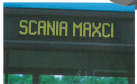
The route number and destination board is integral with the body side.
