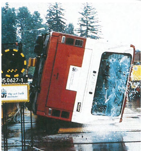
The Scania MaxCi is built from stainless materials. The body frame is of stainless steel - strong, light, durable and easy to repair. Other materials includes aluminium and plastic.
